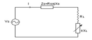
$$P_{L} = I^{2} R_{L} \text{ where } I = \frac{V_{S}}{(R_{S} + R_{L}) + j(X_{S} + X_{L})}.$$
