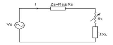
$$P_L = I^2 R_L = \left(\frac{V_s}{Z}\right)^2 R_L;$$
