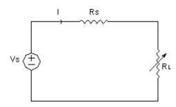
For this circuit the power absorbed by the load resistance 'R<sub>L</sub>' is,  $P_L = I^2 R_L$  where  $I = V_S / (R_S + R_L)$
